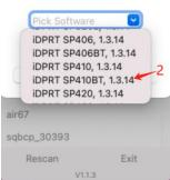
**step2**- Click the "SP410BT-\*\*\*" on the printer list on the tool to connect it.
